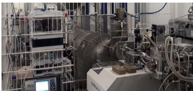
Figure 1 | The beamline P12 at EMBL Hamburg allows studying the structure of molecules in solution using small-angle X-ray scattering (SAXS) technique. (Svergun group/EMBL)
