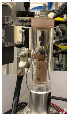
Figure. Compact load frame used to for the in-situ loading and heating 3DXRD, SAXS and tomography experiments. Joule heating are utilized for heating the sample.
